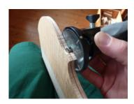
2) I use a small electric saw to cut the edge to the thickness of the finished corners and button. This saw can be used very precisely, owing to its small size and the large surface that rests against the plate. The thickness of the plate will depend on the depth of the fluting and the radius of the gouge — I generally cut it to 4.7 mm.
