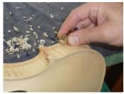
**7)** To finish off the outlines, I prefer to use a flat thumb plane for the bouts and a knife, plus a range of different files, for the inner curves.
