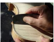
**9)** I cut the fluting almost all the way to the edge (leaving around 0.2mm) and cut down the purfling. Next, I work on the transitions to the arching and scrape arching. I scrape to the edge again (as described in step 4) without worrying about damage to the edge, as any mistakes will disappear when the edges are rolled over.
